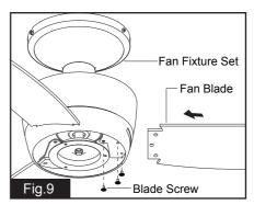
Insert the fan blade through the slot on the fan fixture set. and fasten fan blade to the fan fixture set with screws. Repeat for remaining fan blades.
