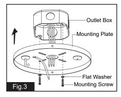
Screw the safety cable hook to the ceiling outlet box. Insert wires from the outlet box through the hole in center of mounting plate. Attach the mounting plate to the outlet box by using two flat washers and mounting screws.
