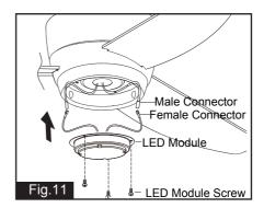
Make wire connection. Plug the male connector from the motor into the female connector from the LED Module . Carefully put the wires into the switch box. Secure the LED Module up to the bottom of the motor with LED Module screws.
