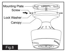
Position both slots on the canopy directly under and in line with two screws and lock washers in the mounting plate. Lift the canopy, allowing the two screws and lock washers to slide into the mating slots. Rotate the canopy counterclockwise until both screws from the mounting plate drop into the slot recesses. Tighten screws securely. Install the other two screws and lock washers into the mating holes of the mounting plate and tighten to secure the canopy to the mounting plate.
