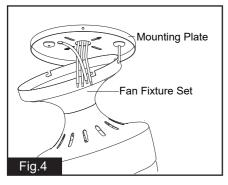
Left fan fixture set and hang on mounting plate with hook provided, through one of the two holes in canopy. This will allow for hands-free wiring.
