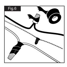
Twist wire ends together and screw wire connectors on in a clockwise direction. tape wire connectors and wire together. instructions that the splics after being made should be turned upward and pushed carefully up into the outlet box.
