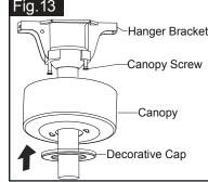
Slide the canopy up to ceiling and over the two canopy screw on hanger bracket. Rotate canopy clockwise, next, while holding the canopy with one hand, slide the decorative cap over the screws and rotate clockwise until tight.
