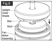
Secure the uplight outer shade onto fan motor assembly by aligning studs and slots, and turn clockwise until it is locked in place.
