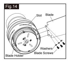
Insert the blade into blade holder according slot then tighten blade to blade holder by using blade screws and washers.
