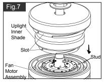
Secure the uplight inner shade onto fan motor assembly by aligning studs and slots, and turn clockwise until it is locked in place.
