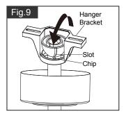
Hang the fan on hanger bracket, and make sure the slot of hanger ball is snapped into the chip of hanger bracket exactly.
