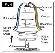
Thread the motor wires through the uplight inner shade, uplight outer shade, decorative cap (Making sure the smooth side of decorative cap is facing downward.), canopy and downrod.
