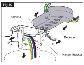
Move ground wires (a), outlet box wires (b), and motor wires (c) away from the center of the hanger bracket as shown. Thread the antenna through the hanger bracket first, then thread the receiver through the hanger bracket until it is placed in the center. Finally, cut motor wires (c) to length needed for connections.
